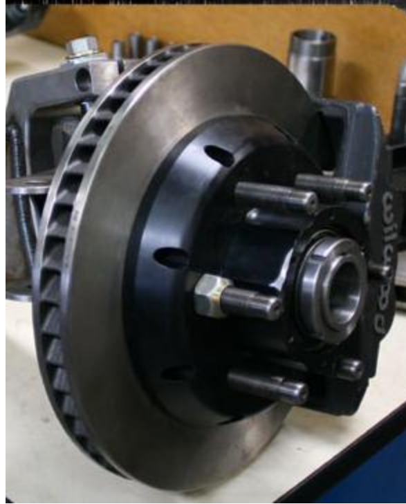
Figure 3.4.4 -- Rotor with cooling vanes (Brake Rotor)
