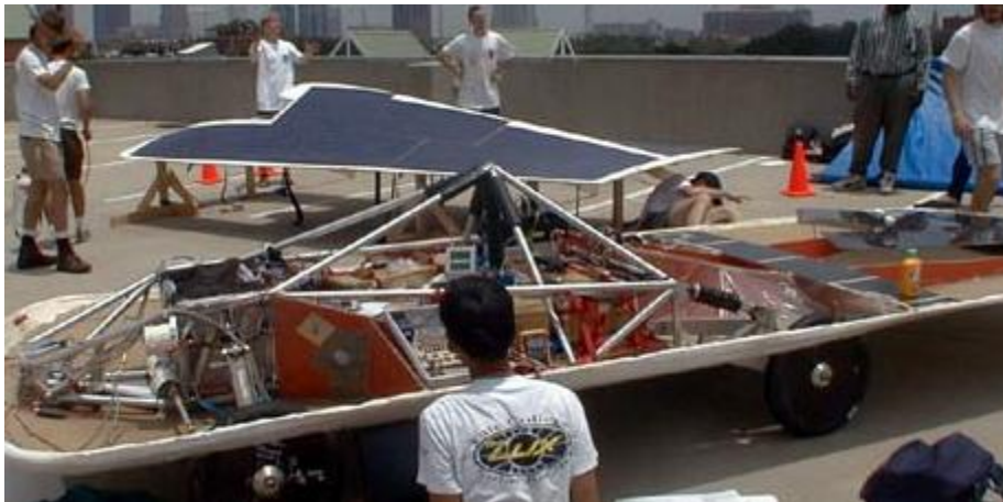
Figure 3.1.4---Aluminum Frame with Outer Shell (Cyber, 1999)
